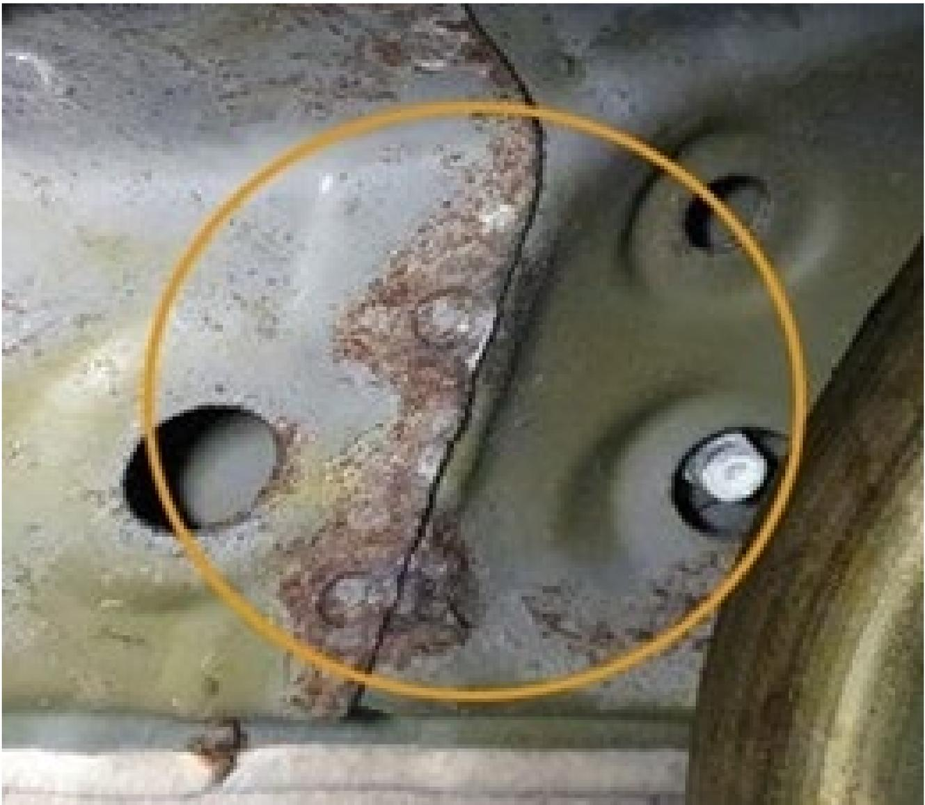
**Image 2:** loose/flaking rust scale has not been removed and is still present.
