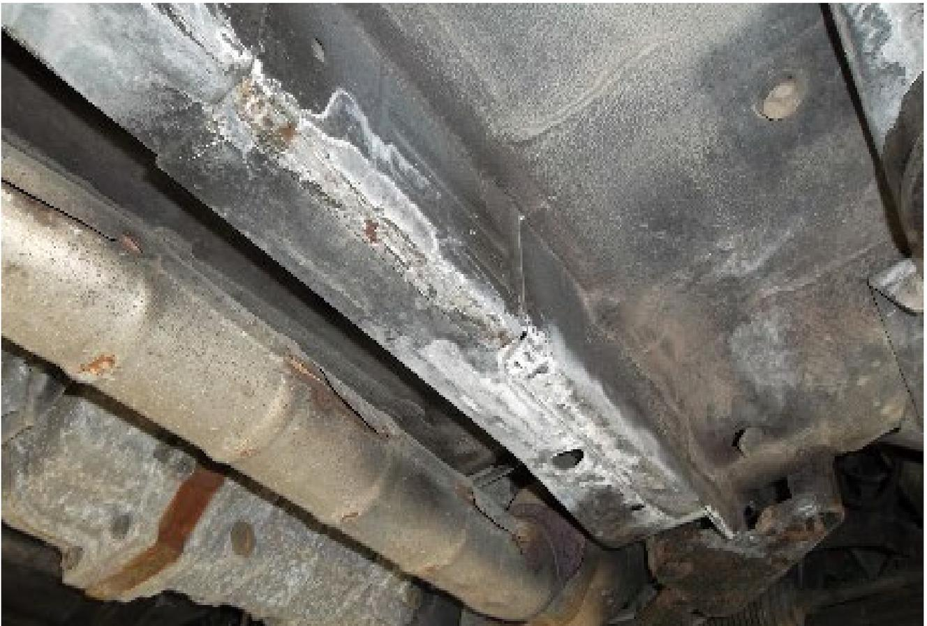
**Images 4:** the dry phosphorous coating created by the acid reaction to the metal (the white, powdery coating seen on the surface), is detrimental to the adhesion of subsequent topcoats.
