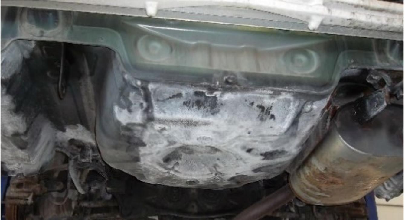
**Image 1:** example of Acid Wash unnecessarily applied to a non-rusted surface.
