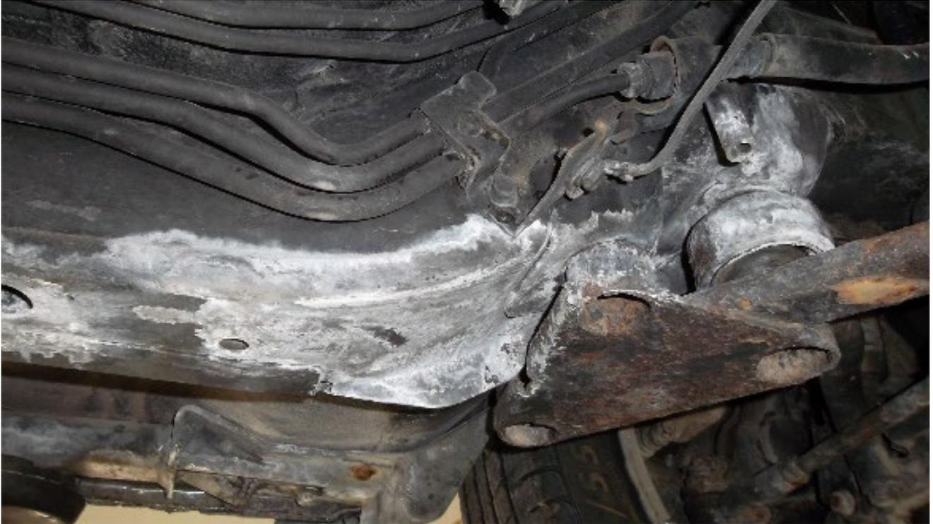
**Image 3:** very little iron oxide (rust) is neutralised/removed when acids are indiscriminately applied and not properly worked into the surface.
