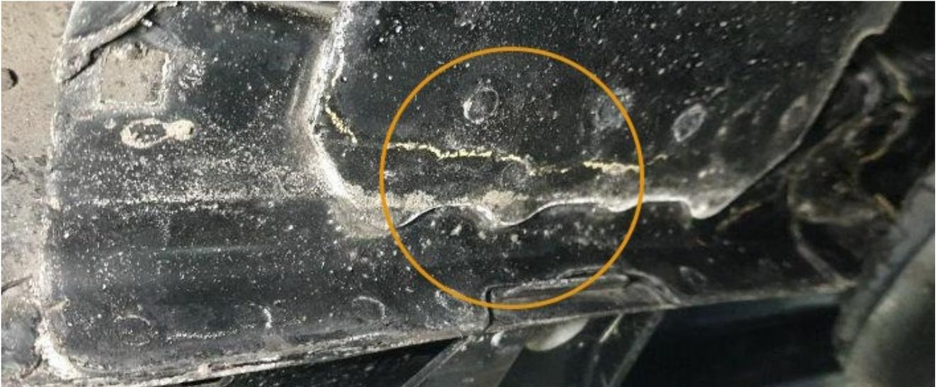
**Image 5:** acids not neutralised/removed (especially in difficult to access areas e.g. the inside of box sections and welded seams), can continue to attack any exposed metal surfaces, breaking down or degrading other protective coatings that they come in direct contact with, and allowing further corrosion to develop.
