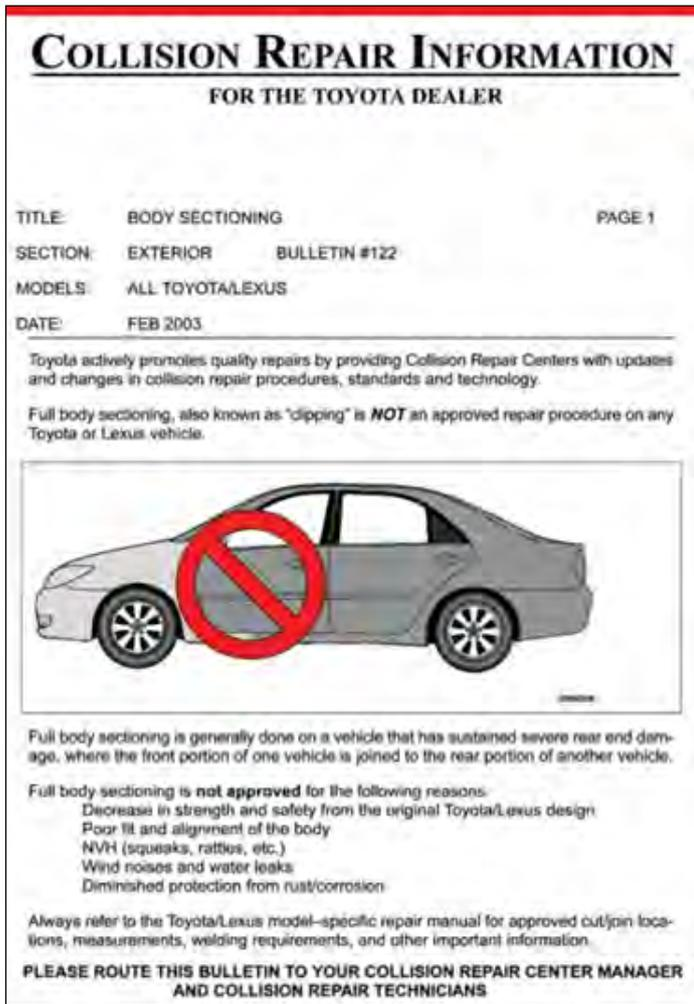
Image 4: Collision Repair Information (Toyota CRIB #122 – Body Sectioning).
