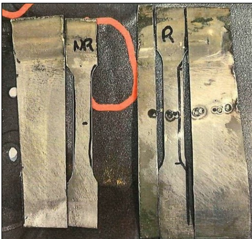
Image 6: The tensile strength sections have been roughly cut to shape from the 'R' and 'NR' samples.
