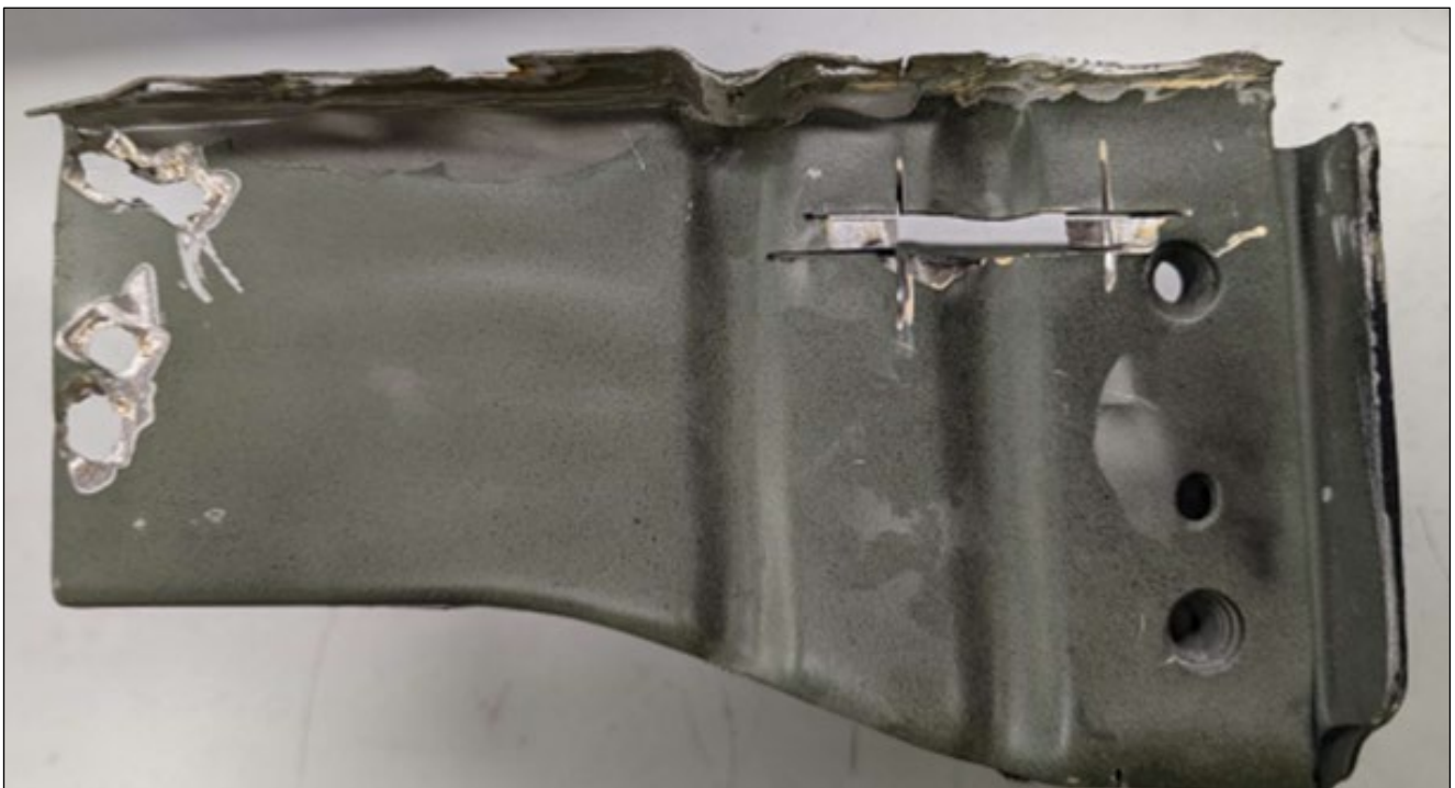
Image 3: The removed damaged and repaired rail section, prior to fitting a new part. The 'slot' cut from the removed section enabled a preliminary inspection of the material to take place.
