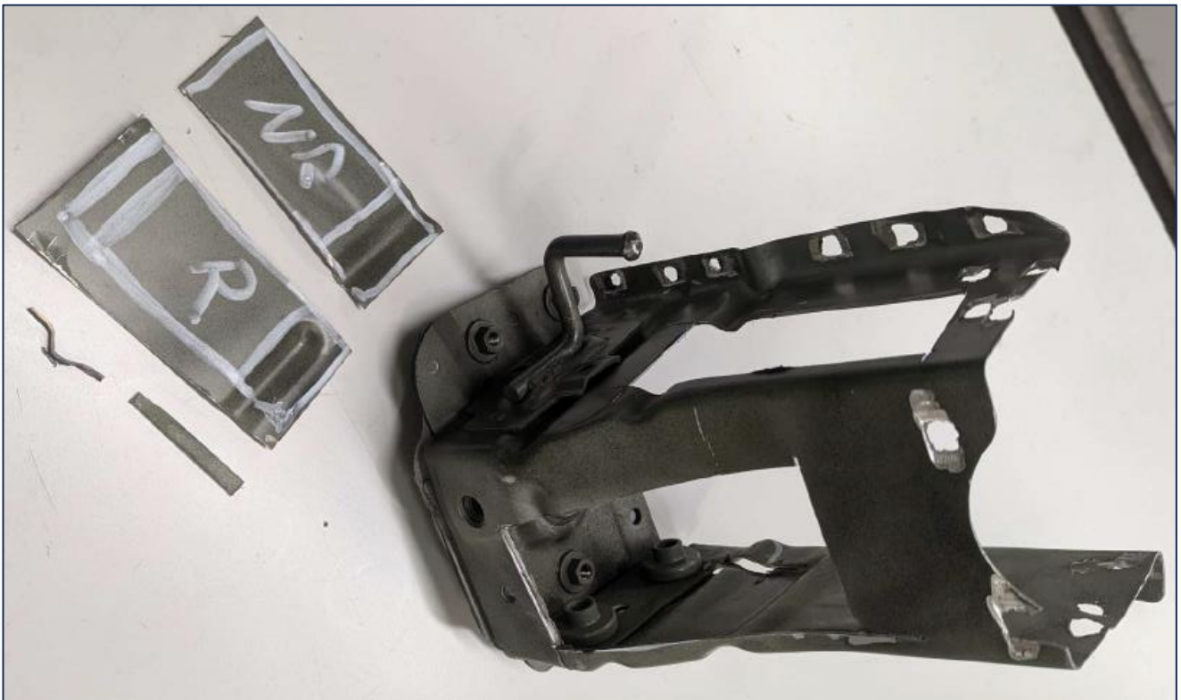
Image 5: This photograph shows the extracted samples cut from the chassis section, and marked 'R' (Repaired), and 'NR' (Not Repaired).
