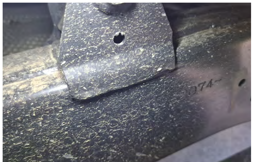
Image 1: Shows the view through a hole in the chassis rail. Image 2: Shows grinding marks on the bracket (hard to see, even in a close-up).
