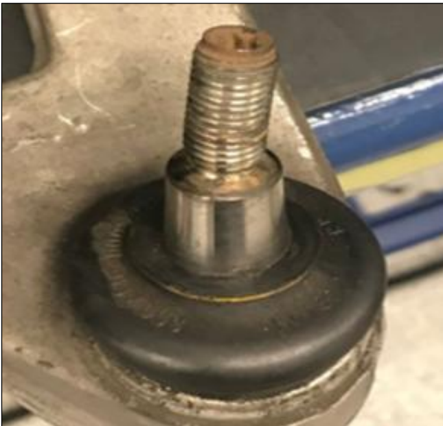
Image 20: Bent ball joint threaded shaft.
