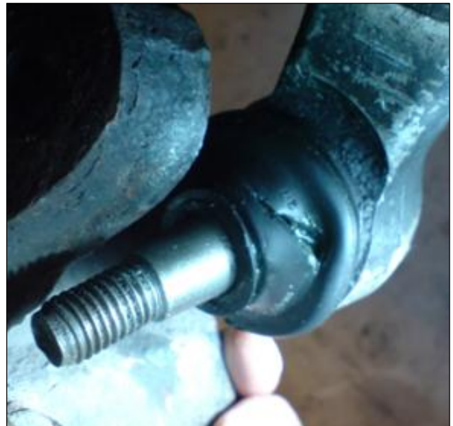
Image 21: Protective rubber boot damage.
