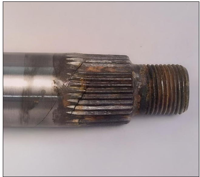
Image 31: Example of a cracked and twisted sector shaft.
