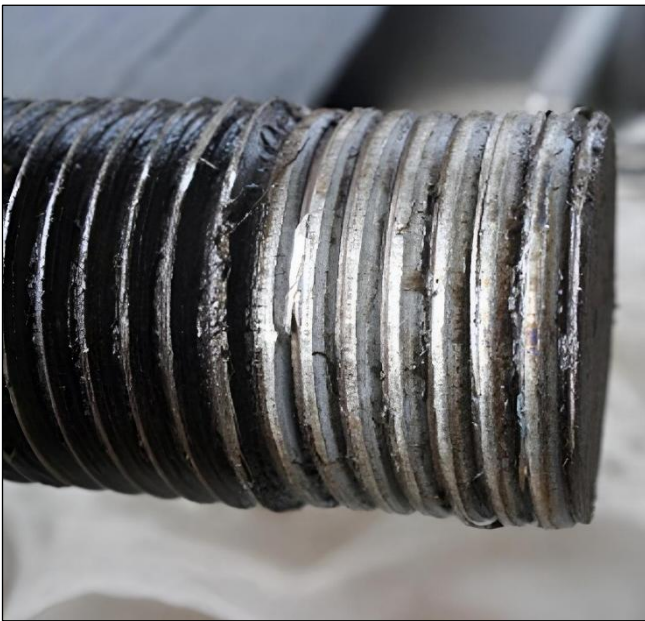
Image 18: Distorted and stripped the threads.
