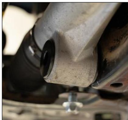
Image 13: Example of mounting bush damage.
