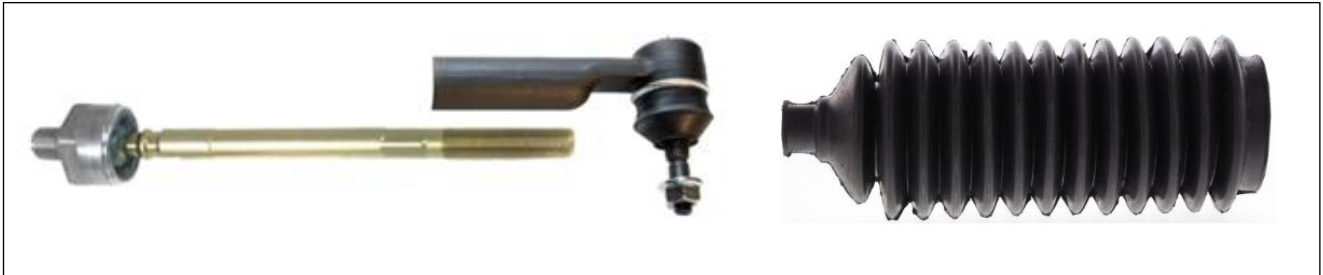
Image 8: Inner and outer tie rod end components.
