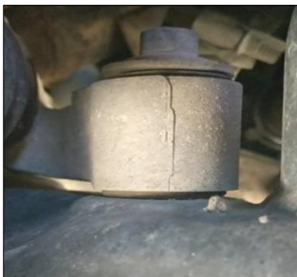
Image 12: A cracked steering rack mounting lug.
