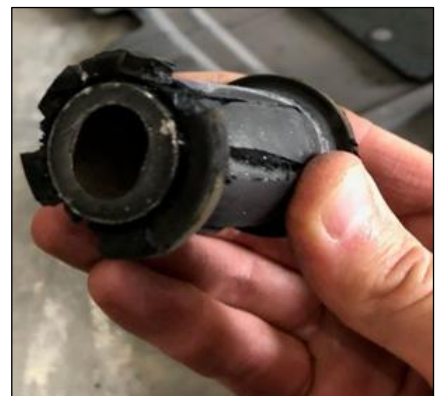
Image 14: Example of mounting bush damage.
