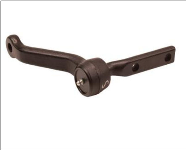
Image 27: Typical example of an idler arm.
