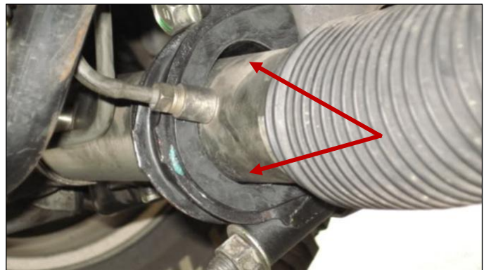
Image 11: Bent or distorted mounting points and mounting hardware.
