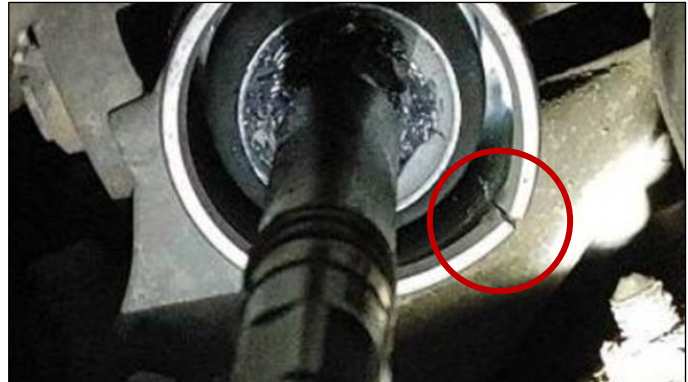
Image 10: A crack/fracture in the steering rack housing.
