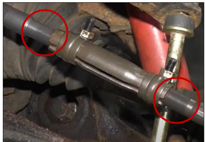
Image 24: Tie rod ends correctly installed into the adjusting sleeve (evenly adjusted and securely clamped). Note the correct positioning of the clamps on the adjusting sleeve.
