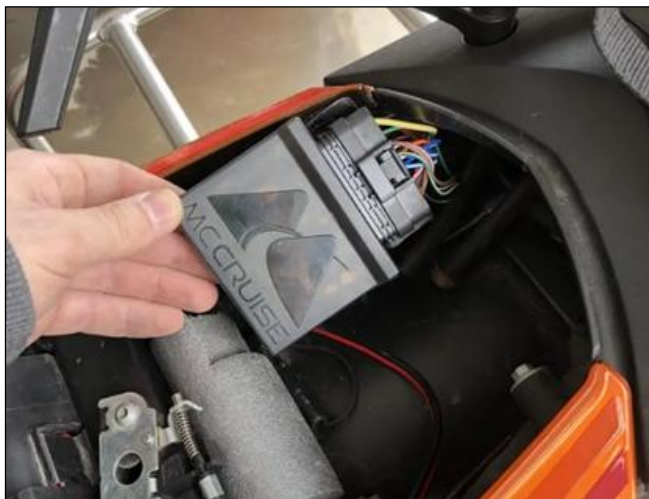
Image 5: An electronic control unit (ECU), located under the seat in this example ( Image credit 4 ).
