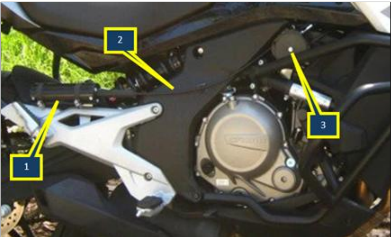
Image 8: Electric throttle servo motor (1) connecting cable (2) Cable Interface Unit (CIU) or 'Spool' (3) (Image Credit 6).
