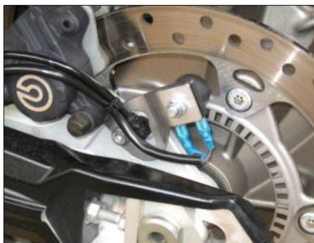
Image 6: Example of an aftermarket speed sensor and mounting bracket, with the pick-up magnets attached to the brake disc bolts ( Image Credit 5 ).
