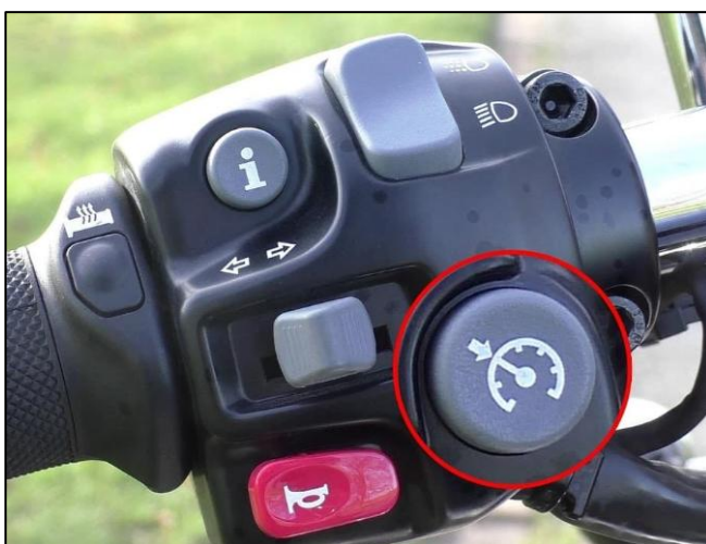
Images 3 and 4: Examples of control switch arrays used on different electronic cruise control systems; an OE unit at left (Image Credit 2), and an aftermarket unit at right (Image Credit 3).
