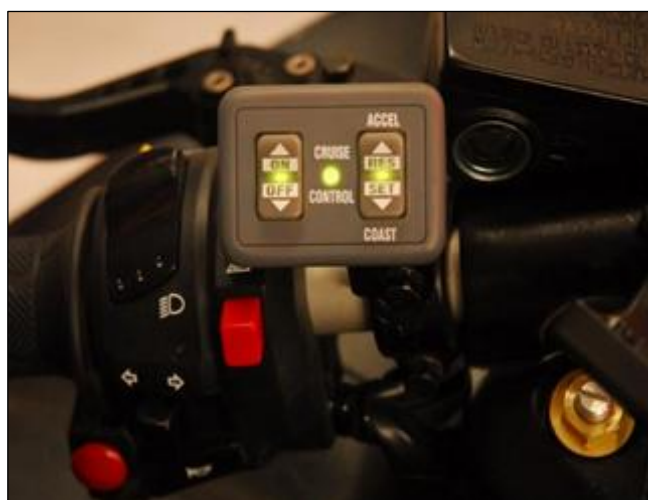
Images 3 and 4: Examples of control switch arrays used on different electronic cruise control systems; an OE unit at left (Image Credit 2), and an aftermarket unit at right (Image Credit 3).
