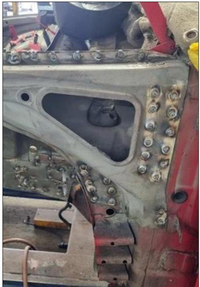
Image 20: Upper inner guard reinforcement to A-pillar weld points.
