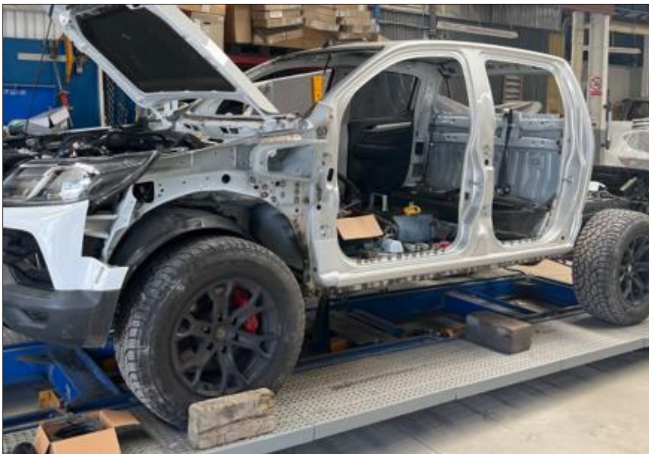
Image 12: The complete inner and outer body-side aperture sub-assembly (including the roof) is replaced.
