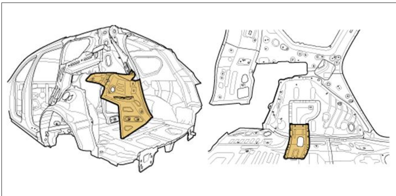
Image 33: In this example, the inner rear quarter multi-panel sub-assembly doesn't include the two components shown in yellow.
