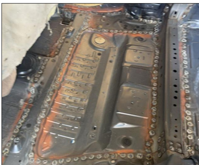
Images 10 and 11: In these further examples of what must not be done, adjacent welded components have been either fully removed (Image 10), or sectioned (Image 11), to access the inner weld points.
