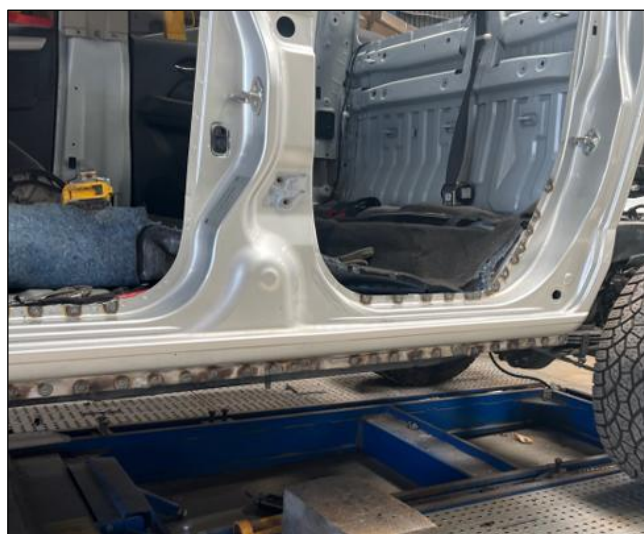
Image 14: Weld point detail - sill and C-pillar.
