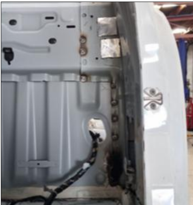
Images 5 and 6: Many of the required weld points are in concealed locations (behind trims, floor coverings, and insulation, etc.) and covered by sealing materials, underseal, or texture coats.
