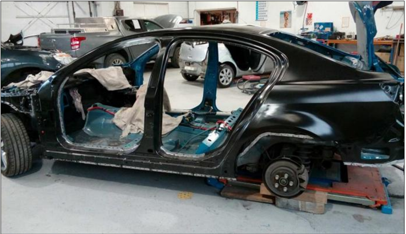
Image 26: The complete (installed) multi-panel body-side sub-assembly on a VF Commodore sedan.
