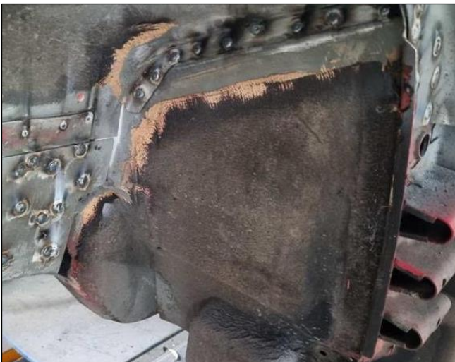
Image 19: Inner guard apron to bulkhead/firewall weld points.
