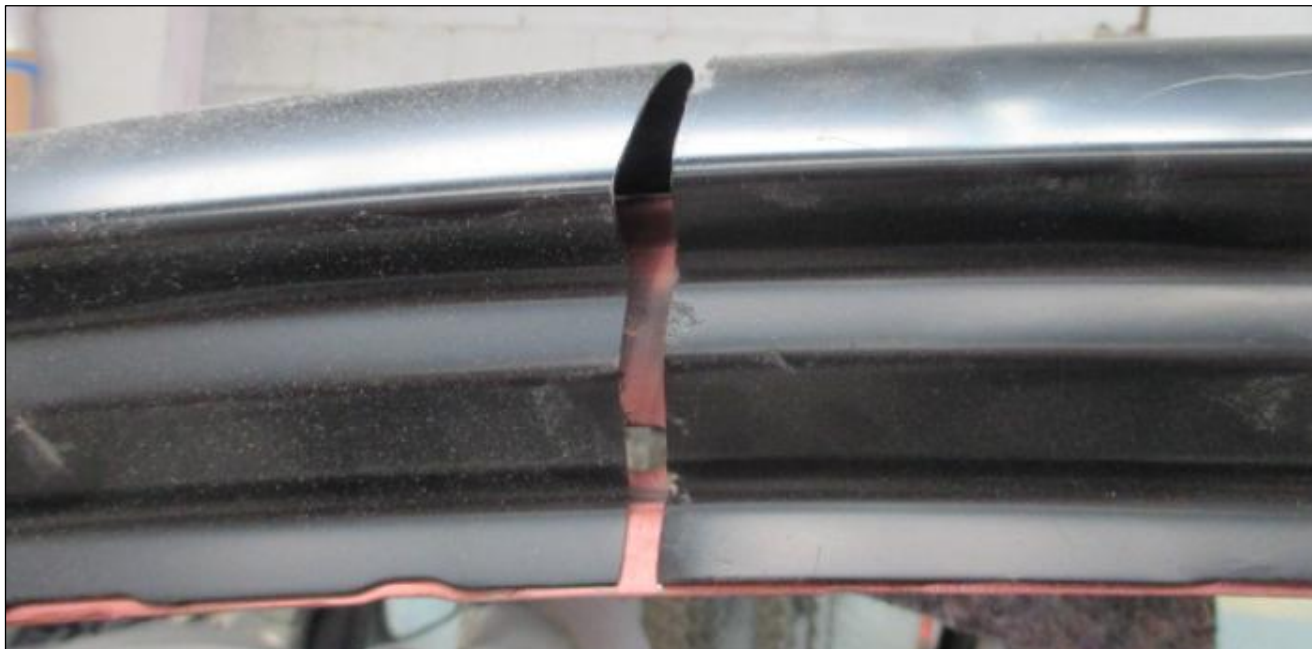
Image 25: When fitting two or more outer panels, the cut locations of the (pre-cut) supply parts often don't match up with each other.
