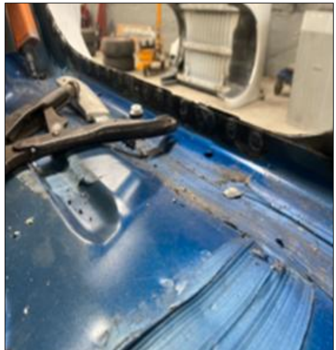
Images 5 and 6: Many of the required weld points are in concealed locations (behind trims, floor coverings, and insulation, etc.) and covered by sealing materials, underseal, or texture coats.
