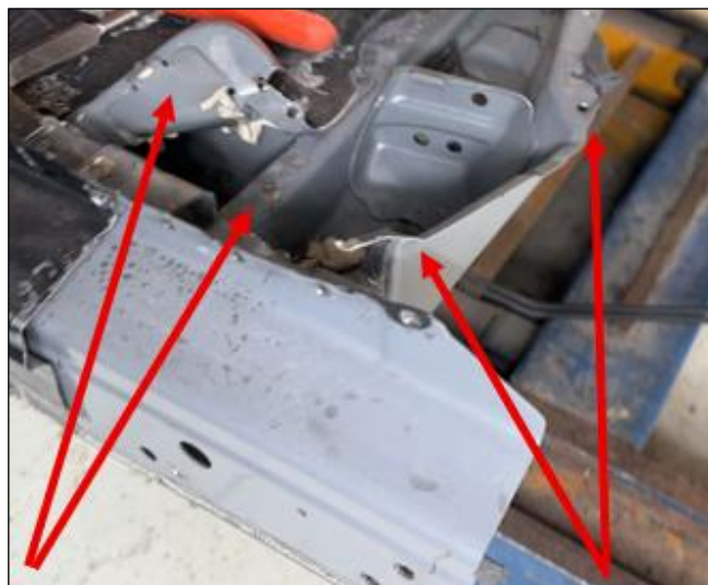
Images 8 and 9: In these examples of what must not be done, adjacent welded components have been peeled back to access the inner weld points.
