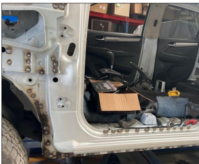
Image 13: Weld point detail - A-pillar and sill.
