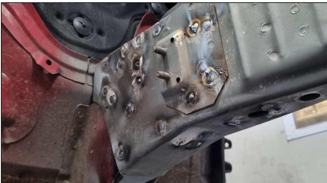
Image 18: Chassis rail to floor-pan rail weld points.
