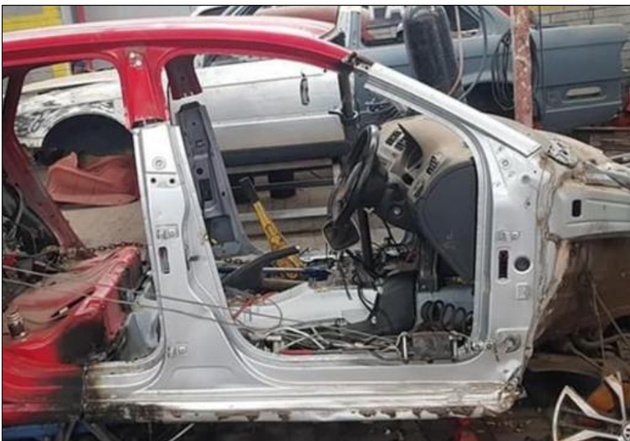
Image 1: A cut and shut example - the major body sections of two vehicles are joined to make one body structure. Image credit (1) .
