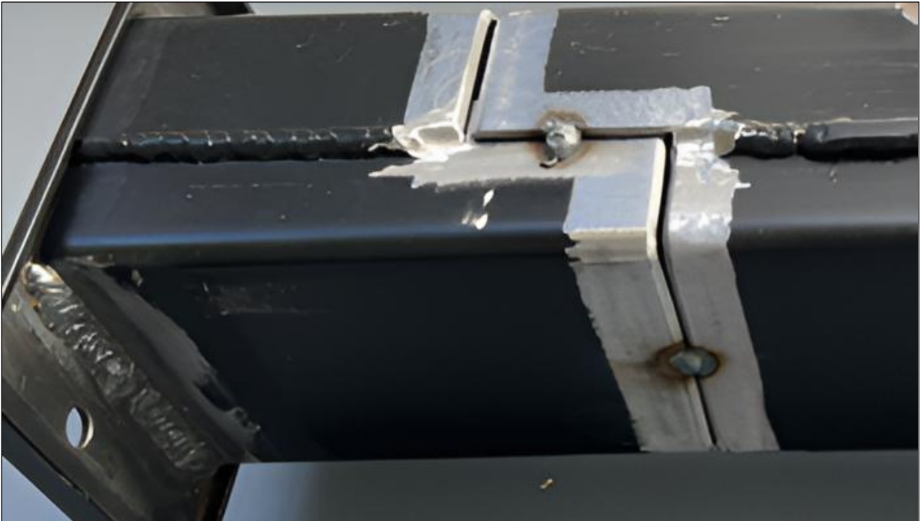
Image 27: Position tack welds away from tight bends and corners (staggered cut joint shown).
