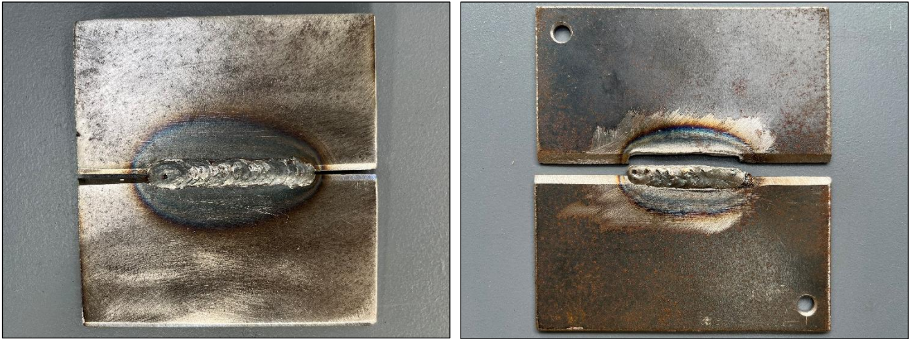
Images 25 and 26: Open-butt joint weld with bevels (single-V layout). The weld bead remains entirely on one coupon, with full length tear out in the other coupon.
