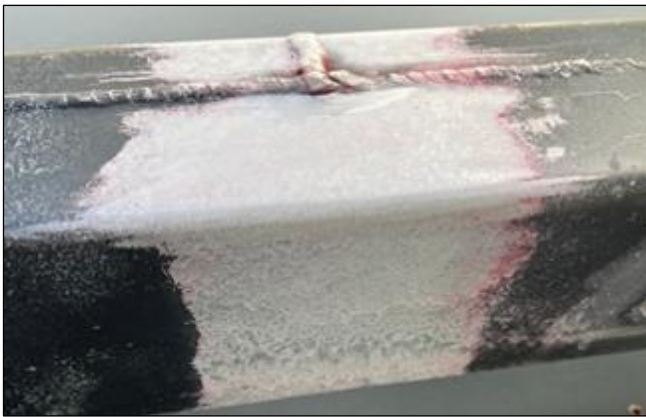
Images 36 and 37: After cleaning off the dye penetrant, the developer draws out the locations of any surface-breaking cracks or flaws.
