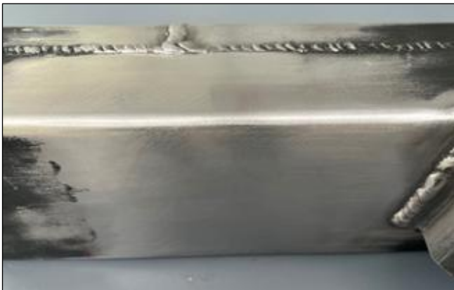
Images 32 and 33: The DPT procedure is completed only after the final surface condition of the weld has been achieved.
