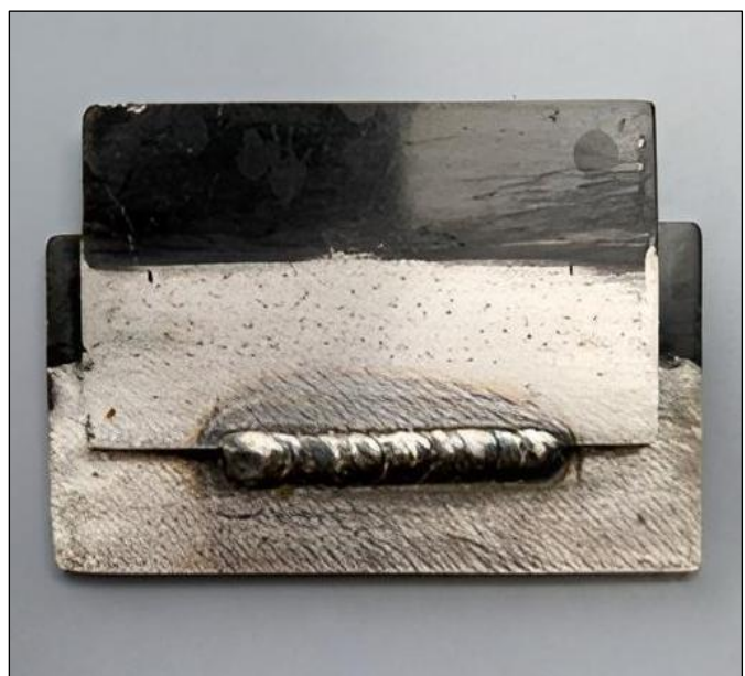
Image 20: The recommended length of practice weld beads is 50 mm.
