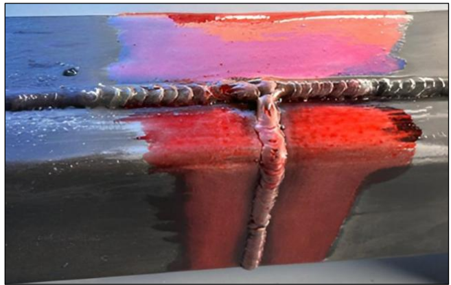
Images 34 and 35: Apply dye penetrant liberally and allow to 'stand' for 10 - 15 minutes (or longer).
