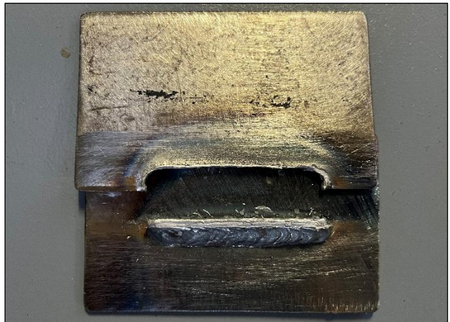
Images 21 and 22: Single-T joint weld (T-fillet). The weld bead remains entirely on the base coupon with full length tear out in the top (vertical) coupon.
