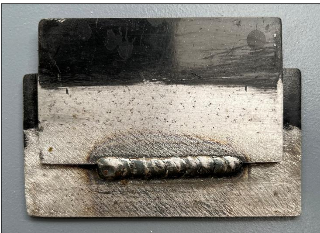
Images 23 and 24: Single-lap joint weld (overlap-fillet). The weld bead remains entirely on the base coupon with full length tear out in the top (overlapping) coupon.
