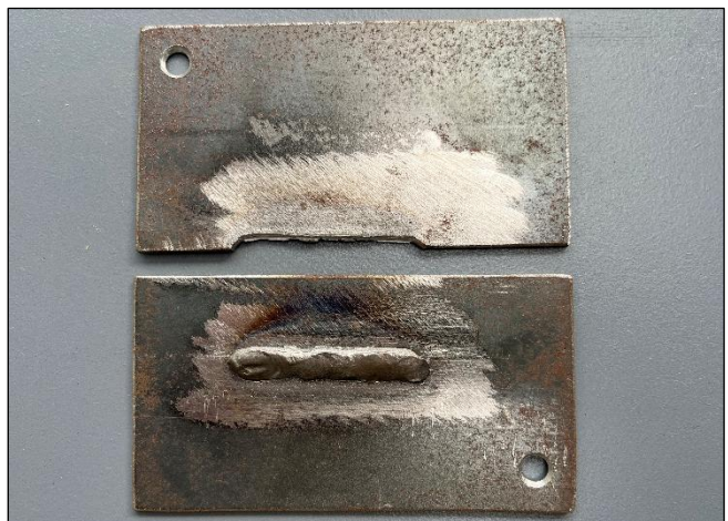
Images 23 and 24: Single-lap joint weld (overlap-fillet). The weld bead remains entirely on the base coupon with full length tear out in the top (overlapping) coupon.
