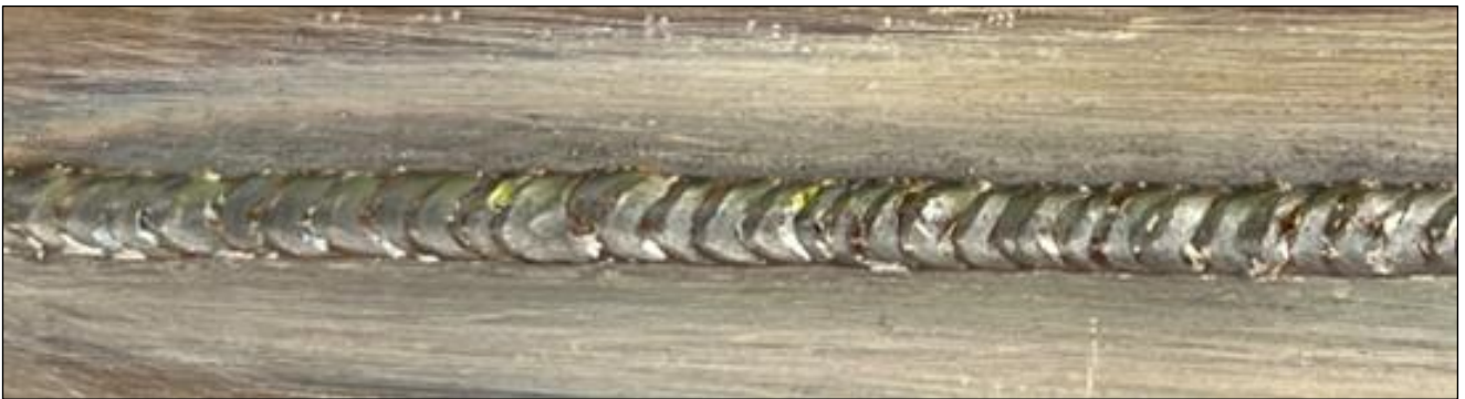
Image 28: Create a continuous weld bead by laying down a series of overlapping 'stitches'.
