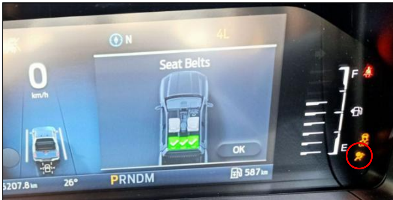
Image 10: Example of SRS MIL self-check system.
