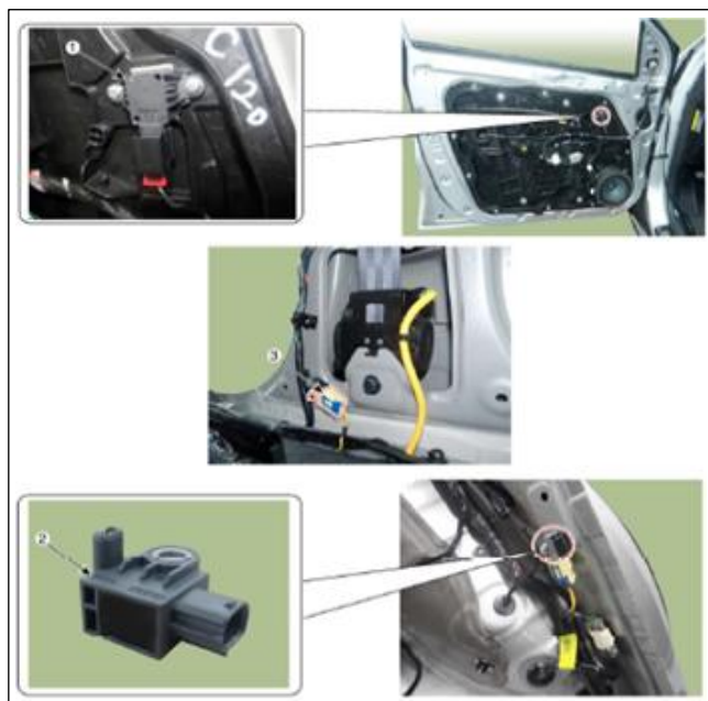
Image 2: Excerpt from a Kia BRM, depicting SRS components and their respective locations.
