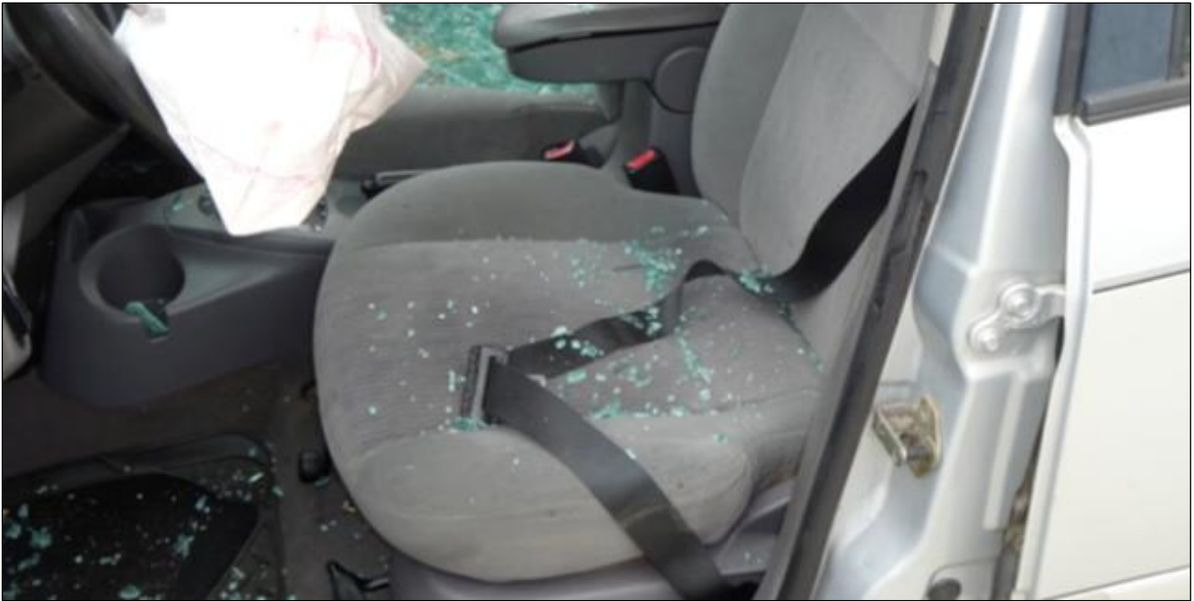
Image 6: A retractor-type seatbelt pretensioner with the belt locked in its extended position (as worn by the occupant).
