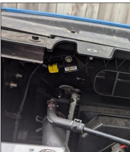
Image 7: Frontal impact sensor (fitted to the radiator core support in this example).
