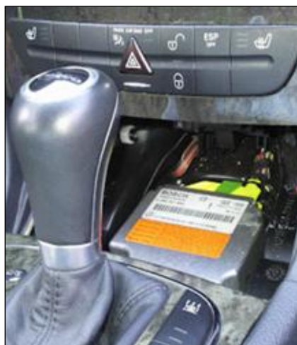
Image 8: Typical location of SRS control modules.
