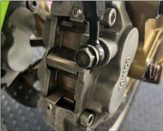
Image 8: Anti-rattle spring plate that typically requires removal.
