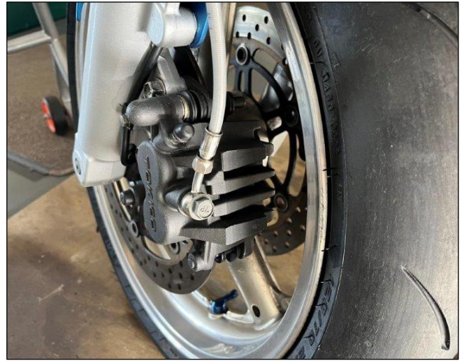
Image 9: Some caliper designs require removal to access the pads.
