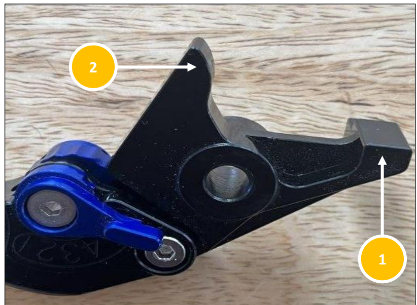
Image 4: Close-up of brake lever return stop (1), and brake actuation lever (2).
