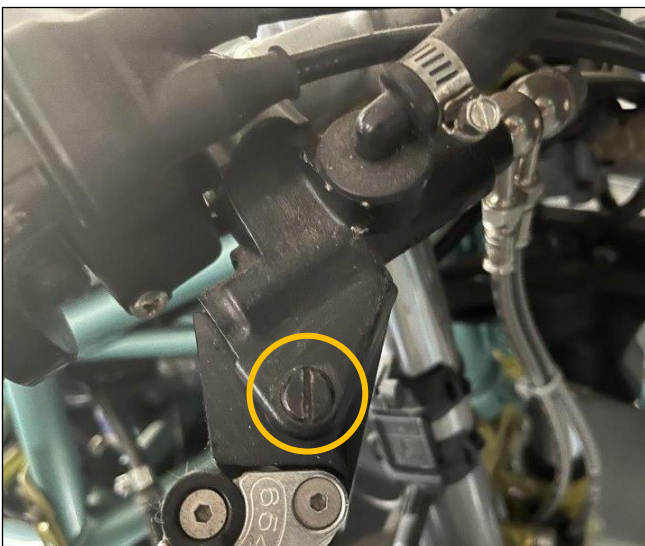
Image 10: Lever-to-perch pivot bolt/pin.
