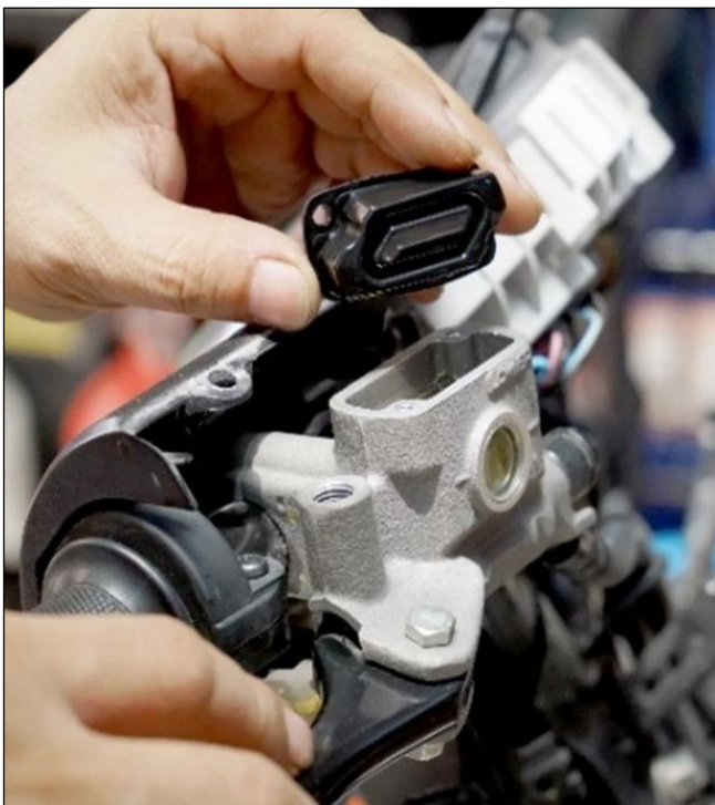
Image 6: Checking for a small fluid pulse inside the fluid reservoir.
