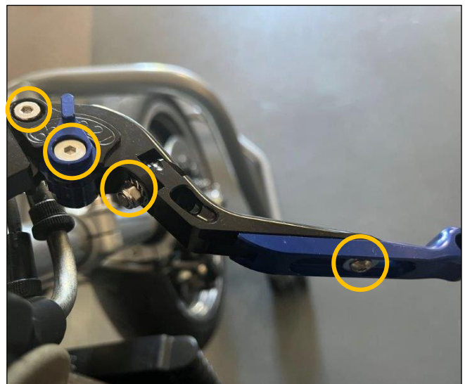
Image 11: Typical adjustable pivot fastener locations.
